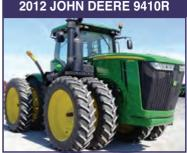
830 Hours. 18/6 PS. Premium Cab. 7" Screen, PTO, 5 Remotes, Hi-Flow Hyd., HID Lights, JD Link, Dual Beam Radar, Guidance Ready, Cat 4 Drawbar, 480/50 Michelin Tires, Factory Warranty November 2015
